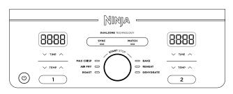
When setting time, the digital display shows HH:MM.
