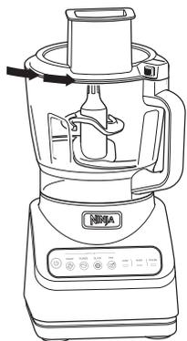
**7** When finished, press the button on the feed chute lid near the handle to unlock, then turn the lid anti-clockwise. Lift the lid from the bowl. Always remove the Chopping Blade Assembly before emptying the ingredients from the bowl. To remove the Chopping Blade Assembly, carefully grasp it by the top of the shaft and lift it out of the bowl.
