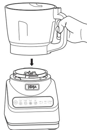
**2** Lower the Food Processor Bowl onto the motor base and rotate clockwise until it clicks into place.
