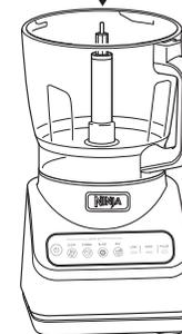
**4** Use the finger holes to grasp the disc and place it over the spindle.
