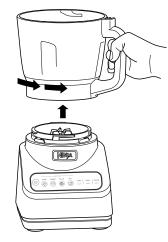
8 To remove the bowl from the motor base, turn the bowl anti-clockwise and then lift it.
