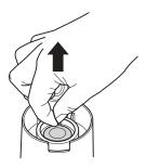
7 Open the flip-top vacuum-seal lid and pull on the green release tab to release the vacuum seal. You will not be able to remove the lid without releasing the vacuum seal.
