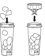
3 Install the Pro Extractor Blades<sup>™</sup> Assembly onto the top of the cup. Twist the lid clockwise until it's sealed tightly. 4 Turn the Single-Serve Cup upside down and install onto the motor base. Align the tabs on the cup with the slots on the base, then twist until it clicks into place. When the unit is connected to power and the container is correctly locked onto the motor base, the program buttons will illuminate and the unit will be ready for use.
