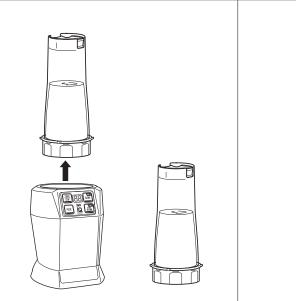
6 When blending is complete, lift the cup up and out of the motor base. Pressure must be released before opening the cup (see step 14 below). DO NOT store contents in the cup with the Pro Extractor Blades™ Assembly attached.
