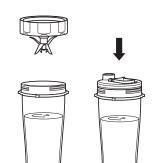
7 Turn cup over so blade assembly is on top. Rotate blade assembly anti-clockwise to remove. To take your blended contents on the go, place the spout lid on cup and turn clockwise to seal.
