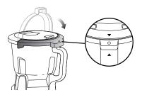
8 Holding the lid by the handle in the upright position, place it on top of the Processor Bowl aligning the triangle ▼ located on the lid with the triangle ▲ located on the Processor Bowl handle. Press the handle down until you hear a click. The triangles on the lid and the Processor Bowl handle MUST be aligned in order for the blender to turn on
